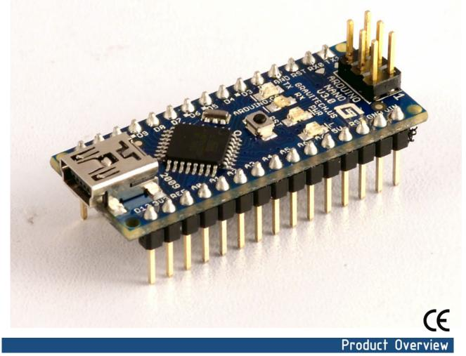
The Arduino Nano is a small, complete, and breadboard-friendly board based on the ATmega328 (Arduino Nano 3.0) or ATmega168 (Arduino Nano 2.x). It has more or less the same functionality of the Arduino Duemilanove, but in a different package. It lacks only a DC power jack, and works with a Mini-B USB cable instead of a standard one. The Nano was designed and is being produced by Gravitech.
