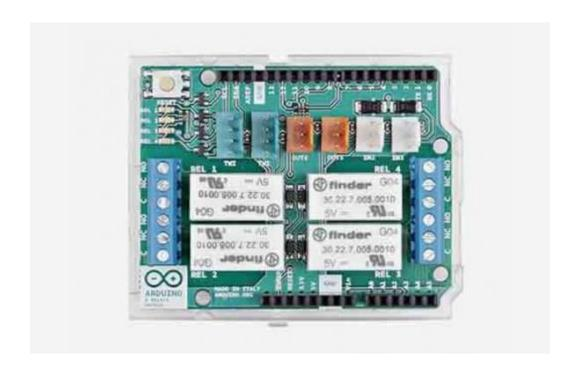
The Arduino 4 Relays Shield allows your Arduino driving high power loads.
