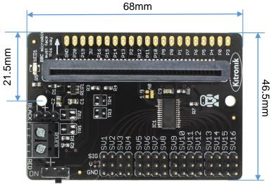
This board conforms to the "Link" standard for accessory boards for the BBC micro:bit.
