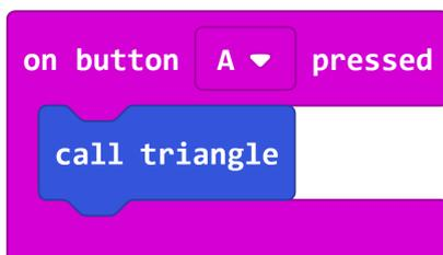
**STEP 4: CODING COMPLTE!** If you have a micro:bit connected, click “Download” to transfer your code and switch on :MOVE Motor. Put :MOVE Motor over some paper, mount a pen and press “button A” to try drawing a triangle.
